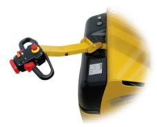
All the control buttons (for traction, lifting + lowering of forks) and slow functions are positioned on the control box
